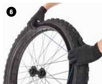
If air is still escaping and the tire beads do not seat on the rim, knock the beads back entirely into the rim channels and add another Inflatoband to each side, totaling 2 per side.
