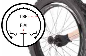
Place the rim "inside" the tire then begin to snap one side of the tire beads into their nearest bead channel.
