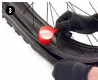
Snap 80% of the second bead into its channel. Add a minimum of 6oz of sealant inside the tire to ensure full sealant coverage.
