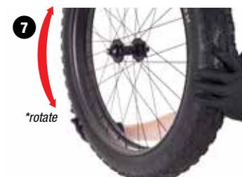
Once the tire is entirely in place, return valve core if removed. Hold the wheel vertical and start with the valve at the bottom. Shake wheel fore and aft to slosh sealant into the bead of the tire. Rotate wheel clockwise after each shaking to seal all potential leaks.
