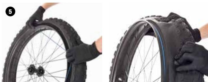
For a tighter seal during inflation, slide Inflatoband into bead channel after the tire bead is in place. Position it so that it does not contact the bead shelf at any point. Inflatobands on the shelf can prevent the tire from sliding into place, and disrupt the air seal. Inflatobands are for mounting only. They remain in the rim but should not be visible once the tire is mounted.
