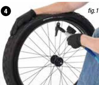
Inflate the tire; between 8-15 PSI, the tire beads will begin to push up onto the bead shelves. If there is a problematic area, step on the leak while applying pressure to the top of the tire with your forearm (step 4 fig.1). Several loud pops are typical as the tire moves into place.
