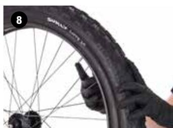
Deflate the tire to the manufacturer's recommended pressure. Double check to make sure that the valve stem is securely tightened to the rim and you're ready to go!
